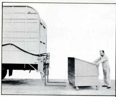
Accumulator equipped with forks so box can be easily removed and left at any location.
