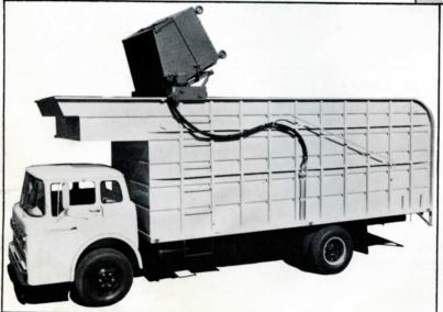
With the use of a lever bucket tilts to dump position.
