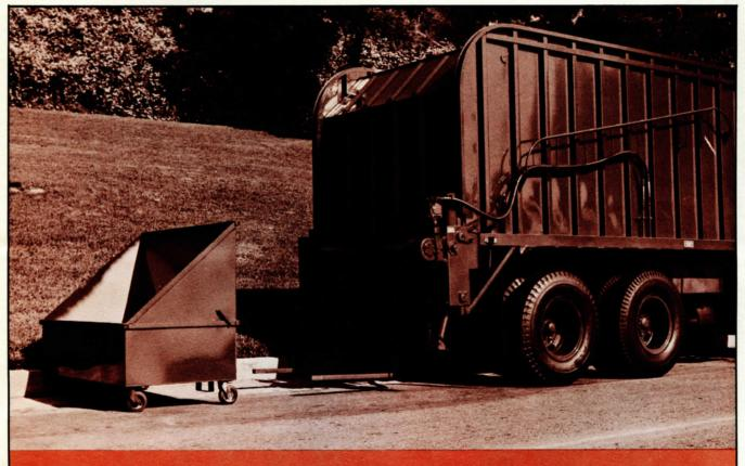
The special loading bin is easily removed and rolled inside buildings for bulk handling of meat trimmings and bones. Low front height of loading bin facilitates easier loading from drums. Lifting
