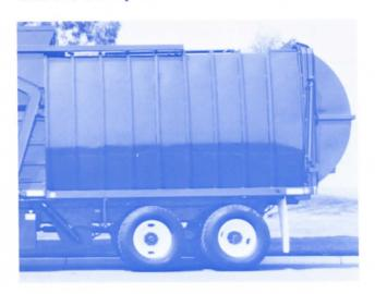
OR a One Piece Hydraulically Accuated Rear Door, single control, fully automatic, all locks are solid weld & never need adjusting. Optional—Rubber Seal.
