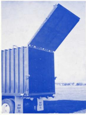
As an option, we offer a one piece Hydraulically accuated rear door with mechanical latches and water-tight seal.
