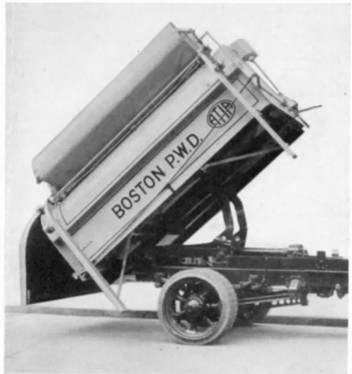
Rear door releases from drivers seat. Dumping angle 45 degrees.
