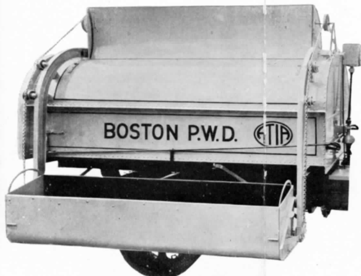
Bucket (9 ft. long x 22 in. high x 21 in. opening across top) lowered to curb ready for load.
