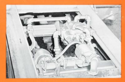
**POWER**— both single-stage ram and telescoping hoist are hydraulically-operated from P.T.O. drive. Simple positive hydraulic pump and valves with electro-vac controls easily and inexpensively maintained. Eliminates extra expense of costly auxiliary chains and motors.
