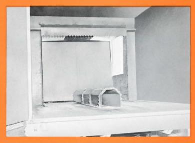
PACKER RAM AND BLADE—single-stage operation for packing as well as "breaking" load for discharge. Ruggedly constructed 3/16" packer blade stays flush with front of body when receiving hopper is being loaded.
