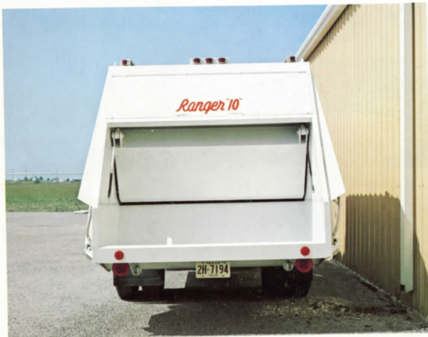
LOW LOADING HEIGHT — 5" below truck frame. Hopper capacity 1¼ cubic yards. Container attachment available.
