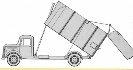
DISCHARGING REFUSE AT THE DISPOSAL POINT This diagram shows the tipping operation; maximum angle of tip is 45 degrees. Note the simple cable hook-up which causes the hinged rear compartment to swing away from the main body when tipping.
