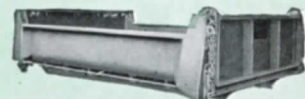
Model 2 —Plain side body for general hauling. 10 gauge high carbon steel, one piece construction.
