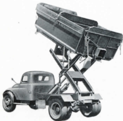
Galion hi-lifts for handling coal. Twin cylinder hoist construction. Special endgate for coal chute optional as an extra
