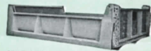
Model 12 —Contractor's heavy duty body with running boards and pyramid side braces for extra strength.
