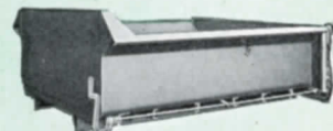
Model 3 —Flared side to permit crowning of load. 75 cubic feet coal body. Front end built high to protect cab. 10 gauge high carbon steel, one piece construction.
