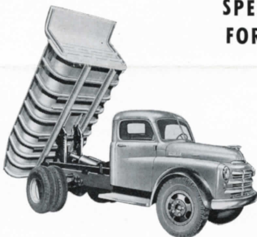
Heavy-duty Boulder Dam type rock body heavily reinforced with wrap-around I-beams. Large cab protector permits loading from shovels.
