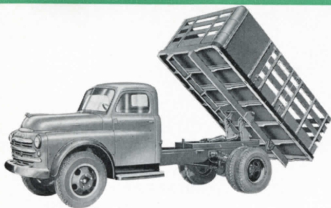
Model GH-567 hoist mounted with platform body for hauling bulk materials. Powered for handling 7½ ton payloads when equipped with a 9 foot body
