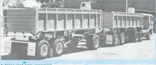
A tipper road train comprising two 24' long 25 cubic yard tipping semi-trailers — one provided with a single axle dolly — was fitted to a Mercedes Benz LPR 2224 chassis for Diesel Coy. (Readymix) Pty. Ltd., account Northern Territory Crushers Pty. Ltd.
