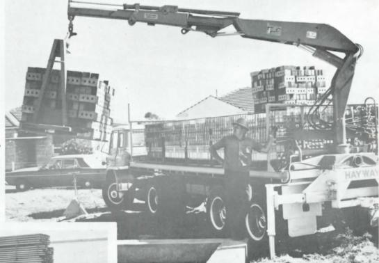
For the carrying of long loads this Leyland 560FG cab has been converted to a half cab to take a GITSHAM 30 foot 'Long Tom' body and a Hiab 173 Speedloader for Port Darwin Motors Pty. Ltd. of Darwin, N.T.
