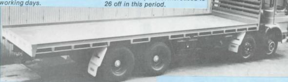
A 28 foot steel framed traybody fitted to an A.E.C. Mammoth Major 250" wheelbase chassis for the British Leyland Motor Corp. of Aust. Ltd. A
