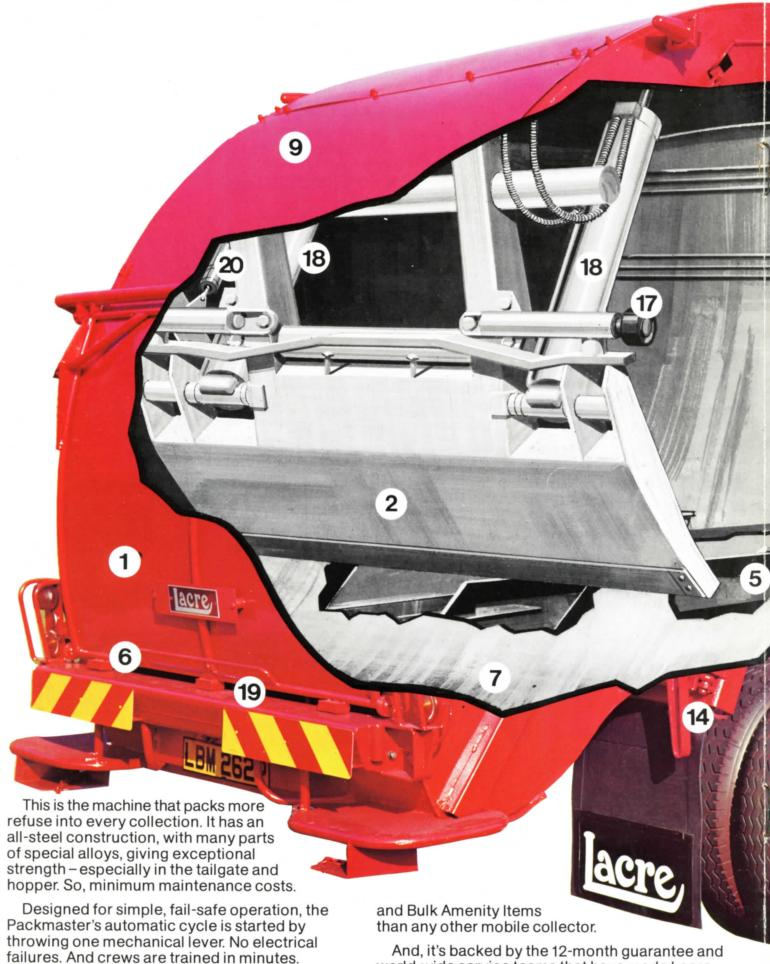
One moving part, the packer plate reaches over the load, crushing, compacting and retaining it. The Packmaster handles a greater variety of Bins And, it's backed by the 12-month guarantee and world-wide service teams that have made Lacre the first choice of Local Authorities, Ministries, Armed Forces, Civil Engineers, Contractors and Industry throughout this century.
