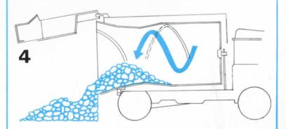
FOR DISCHARGE THE REAR DOOR IS OPENED AND DRUM ROTATED IN REVERSE DIRECTION TO "SCREW-OUT" REFUSE.
