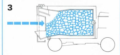
WITH ALL DRUM FREE SPACE FILLED AS LOADING CONTINUES, THE LOAD IS COMPACTED BY THE ACTION OF THE DOOR SHAPE AGAINST THE ROTATING REFUSE.
