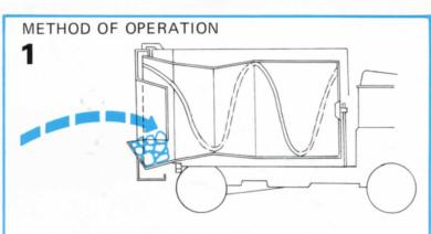
REFUSE IS LOADED INTO THE REAR HOPPER.
