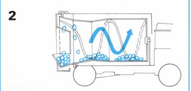
REFUSE IS CARRIED FORWARD, TUMBLED AND BROKEN DOWN BY DRUM ROTATION.
