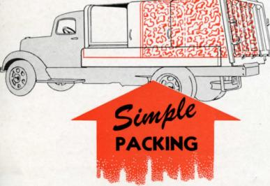
Operating hydraulically, a platen, or packing plate equal to the internal cross dimensions of the body, travels the length of the body. It carries material from the door openings in the front to the rear where it compresses and packs the refuse. This permits the body to be loaded to its full capacity with compressed material. Both the forward and reverse movements of the platen are controlled by a predetermined pressure value and automatic stops.
