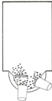
First hopper load displaced forward; second hopper load uncompact
