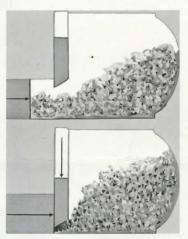
Refuse is first compressed into body by the horizontal ram and is again crushed by the vertical ram, every 20 seconds, thereby providing a high payload density of up to 1,000 lbs. per cubic yard.
