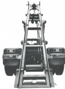
Sani-Haul one truck with fleet capability, payloads to 60,000 lbs.
