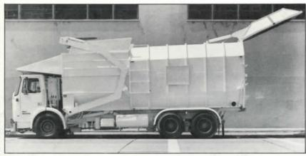
REAR BUBBLE DESIGN DOOR HYDRAULICALLY OPERATED OPEN FOR DUMPING POSITION.
