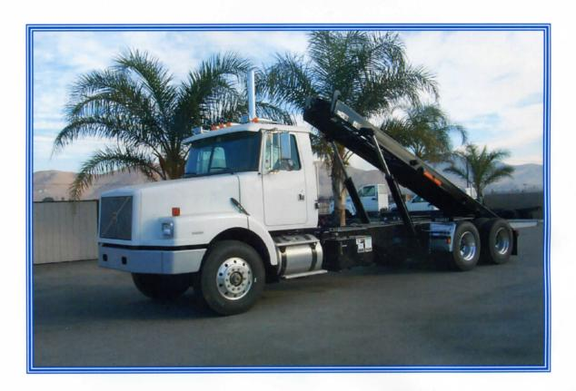
The Amrep Roll Off is a 22' Reeving or Winch type unit with 30,000 lb. line pull capacity. A dump angle of 46 degree with a container capacity of up to 24' is standard. Top channel rail systems are available upon request. Your choice of full or quarter fenders are provided. See detail specification sheet for additional information or optional equipment.
