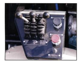
For safety and ease of operations, controls are conveniently situated on the exterior of the vehicle, as well as the center of the cab.
