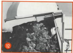
Horizontal ejection, the safest way to dispose of the load. That's important with a "TITE-PAK" load. They're BIG!
