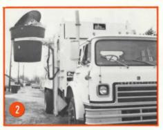
Athey's "CWC" vehicles can handle 80, 90 and up to 300-gallon containers quickly, cleanly, with less expense. Note the level rise.
