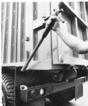
Lever for mechanical hydraulic rear door lock.
