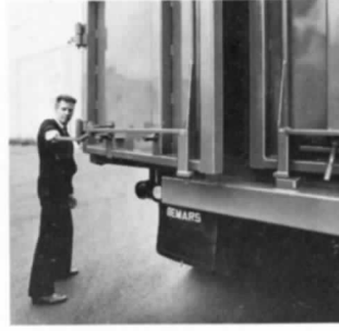
Flush bottom compactor design eliminates rollers.
