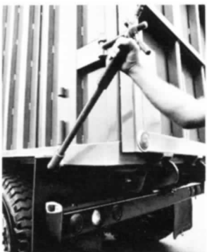
Optional lever for mechanical hydraulic rear door lock.
