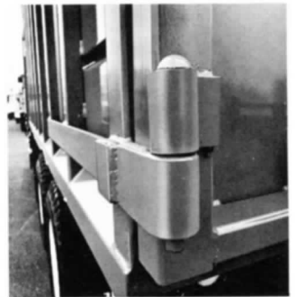
In-turned rear door hinges which offer stronger support to heavily-reinforced rear doors.
