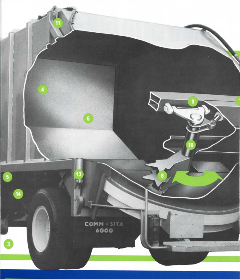
As refuse is emptied into the hopper the rammer packs it against the ejector plate.
