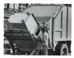
**5500S.** The 5500S has been designed with the growth operator in mind. It is a fully dual purpose refuse machine and will handle 1½ cu. yds. rectangular bins with complete safety and simplicity by single lever operation. The bin lift equipment does not interfere with normal domestic collection.
