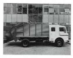
This highly flexible body can be fitted to the majority of perfectly standard chassis cabs either with or without a 6-7 man crew cab.
