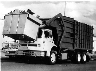
FRONT LOADER OPERATION FOR DUMPING CONTAINERS.
