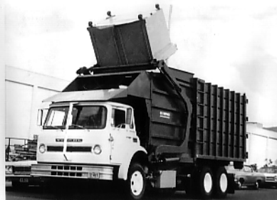
FRONT LOADER OPERATION FOR DUMPING CONTAINERS.
