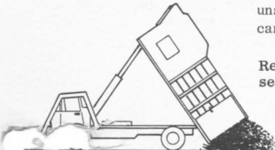
LIGHTER BODY WEIGHT AND FRONT-MOUNT CYLINDERS GIVES BIGGER PAYLOAD WITHOUT REAR-AXLE OVER-LOADING
