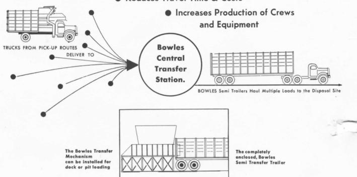
The Bowles Transfer Station principle is designed to reduce the long-haul labor and equipment cost of rubbish trucks going to and from the disposal site. Up to 24 ton legal payloads can be hauled in most states.
