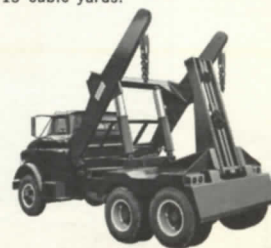
MODEL 1000. This is the toughest Liftainer in the range of standard models and will easily lift a gross load of 24,500 lbs. It handles all sizes of containers up to 15 cubic yards.
