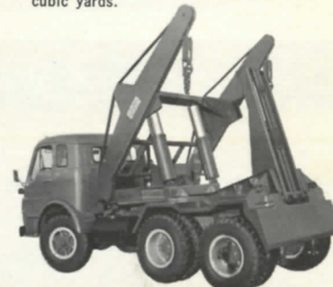
SPECIAL HEAVY-DUTY MODELS. On special order Cobey will provide even heavier units like this Model 1250 built for U.S. Steel Corporation. Special equipment includes 5" stabilizing jacks, and 10" lifting cylinders.
