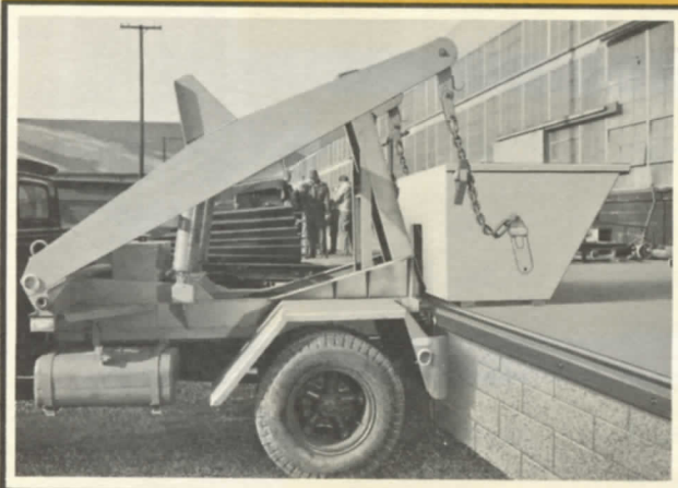
Dock Pickup. Perfection Liftainers can pick up and handle containers from docks 54" high, above-grade positions.
