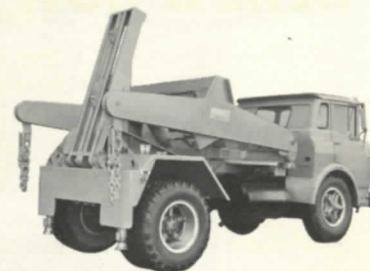
MODELS 160 and 175. Equipped with bigger lifting cylinders these units are built heavier to take loads ranging up to 21,250 lbs. in containers from 2 cubic yards up to 15 cubic yards.
