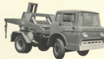
MODELS 140 and 150. These units will handle containers up to 12 cubic yards on all applications and up to 15 cubic yards on other applications. Their gross lifting capacities range up to 13,750 pounds.
