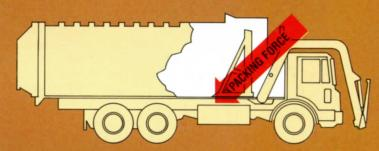
The IFL packing cylinder operates horizontally. All the force is directed into the load not into the floor as with other compaction systems. The result is a 15% increase in effective packing force. Payloads are increased and floor wear is reduced.
