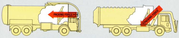
The IFL packing cylinder operates horizontally. All the force is directed into the load not into the floor as with other compaction systems. The result is a 15% increase in effective packing force. Payloads are increased and floor wear is reduced.
