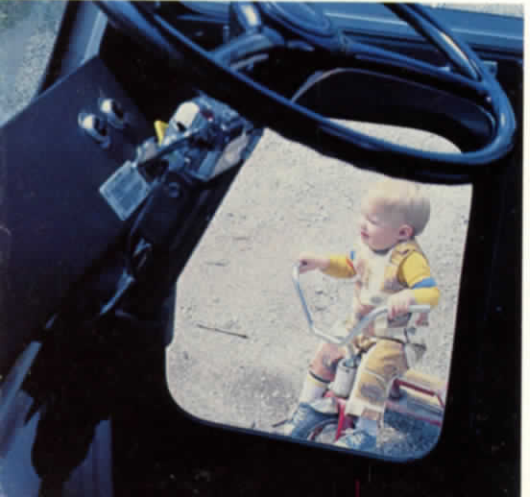
Above: Short step increases productivity Below: Viewing ports eliminate blind spots
