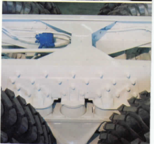
Above: Wide-flanged tandem crossmember Below: Dual controls allow driver to double as collector
