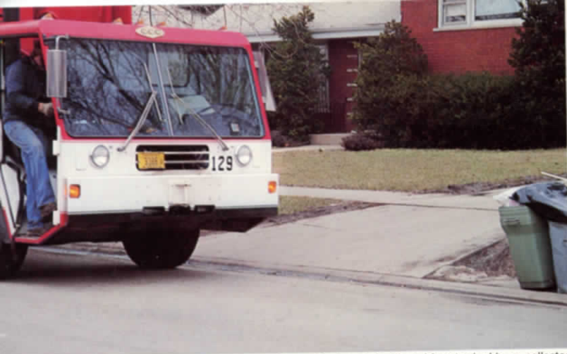
Above: Dual controls allow driver to double as collector Below: Low step height increases productivity
