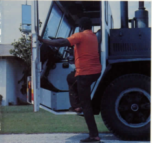
Above: Short step increases productivity Below: Viewing ports eliminate blind spots
