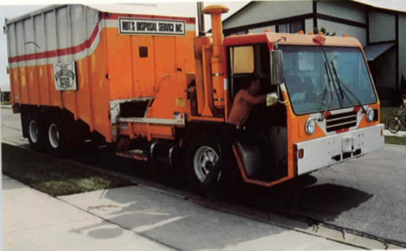
Above: Dual controls allow driver to double as collector Below: Low step height increases productivity
