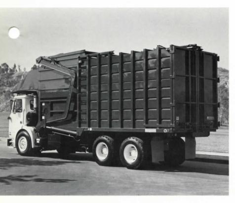
The C&O partial pack, available in 37, 42, 44, and 46 cubic yard models, is a unit designed for speed and efficiency in both commercial and residential applications. A comprehensive list of available features enables the company to manufacture a high quality unit well-suited to each user's specific needs and requirements.
