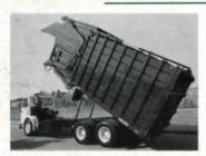
An advantage of the C&O partial pack is the method it employs to unload refuse. The body is hydraulically tilted and the refuse is emptied with the assistance of the eight foot hydraulic packer. This system provides flexibility and ease in maintenance and a quick unloading cycle. The optional hydraulic tailgate makes unloading even faster and easier.
