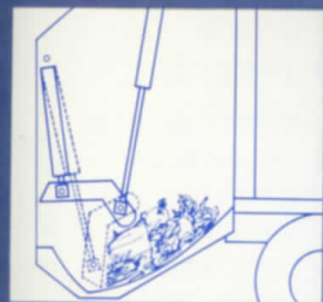
Pre-pack. Blade pre-crushes material against the reinforced hopper floor
