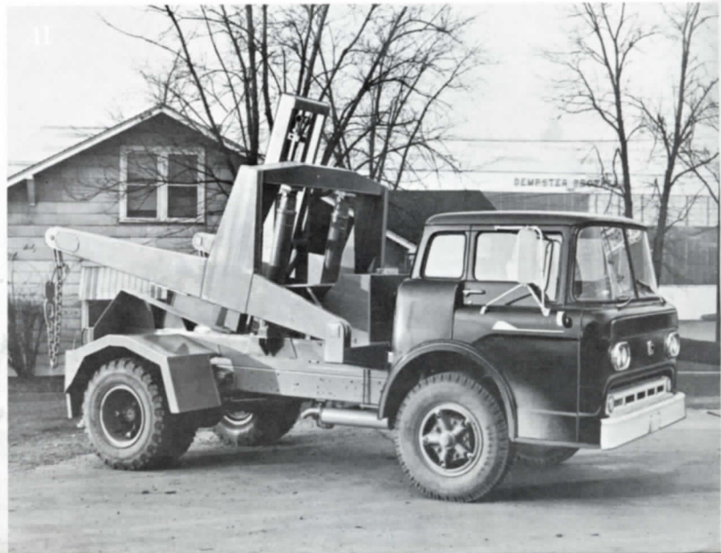
Below, the LFW 403-C Dempster-Dumpster hoisting unit mounted on a conventional truck chassis for all-purpose use.
