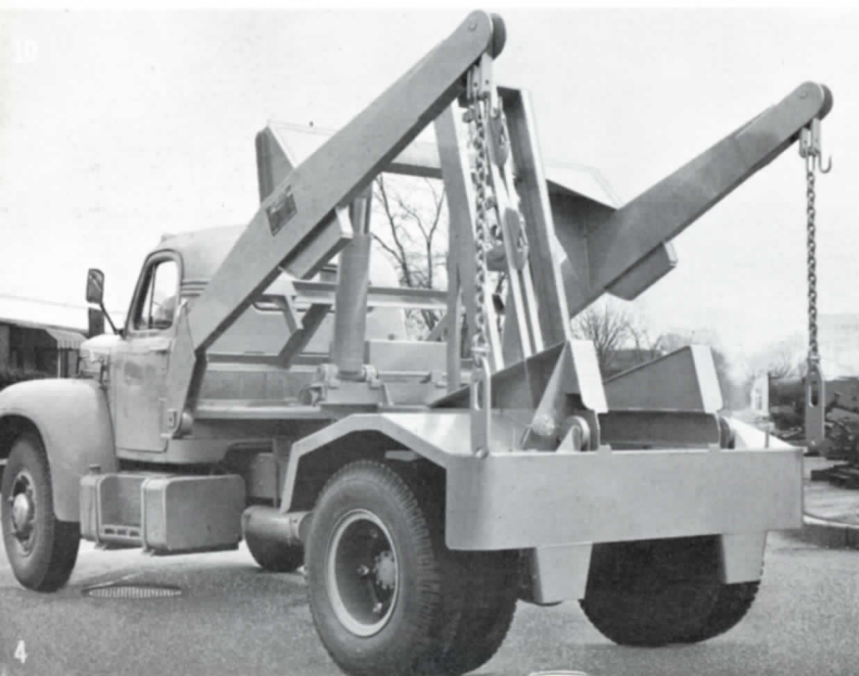
Photo below shows LFW 303-H which is in popular use for handling general industrial waste, with emphasis on dense material in smaller containers.
