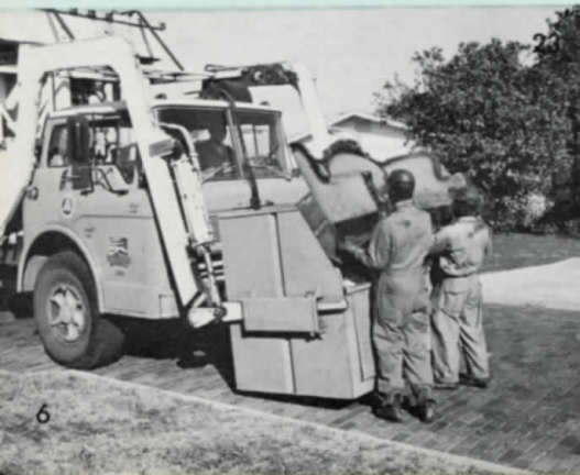
■ Photo 23 illustrates how easily large, discarded household items are accommodated by the container.
