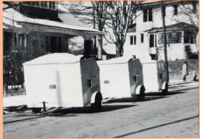
On a residential street in Winston-Salem, North Carolina, three containers have been uncoupled and spaced for emptying operations.
