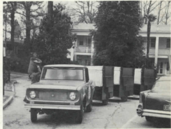
When a container is full, the neoprene/nylon cover is pulled over the refuse and is locked down to prevent escape of any material during transit.
