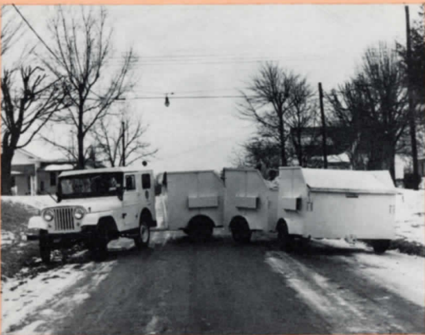
A tight U-turn is negotiated by outrigger type containers, being operated on icy streets in Winston-Salem, North Carolina.
