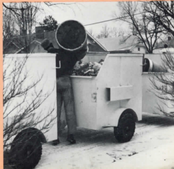
Connecting draw bars space containers efficiently for loading crews to empty refuse from a position between the containers.
