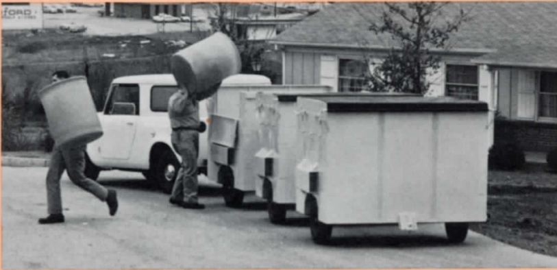
TWO-MAN CREW The size of crew used is determined by the distance of the house from the street, and a number of other factors. Crews range from a driver and three loaders to a driver and one loader. In the two-man system, loader and driver switch off as illustrated in this installation at West Haven, Tennessee.
