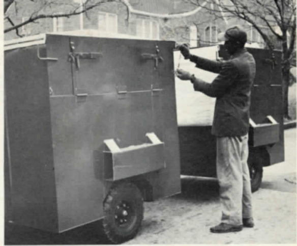
When a container is full, the neoprene/nylon cover is pulled over the refuse and is locked down to prevent escape of any material during transit.
