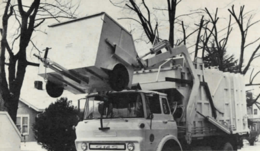
A close-up of a train container just before it is rotated over the hopper of the "Mother Unit" for emptying. The neoprene/nylon cover is released from its moorings but left in place during dumping operations to restrain scattering of refuse.
