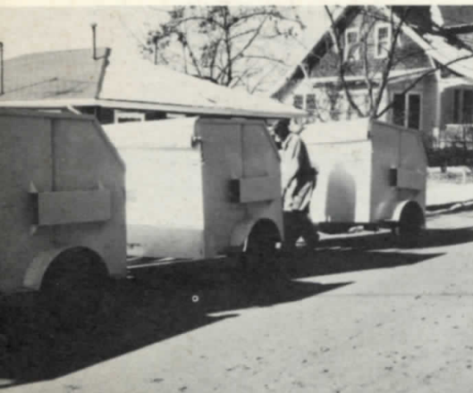
A close-up of a train container just before it is rotated over the hopper of the "Mother Unit" for emptying. The neoprene/nylon cover is released from its moorings but left in place during dumping operations to restrain scattering of refuse.
