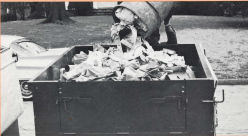
When the refuse nears the top, the side doors are raised so that it may be filled to capacity.
