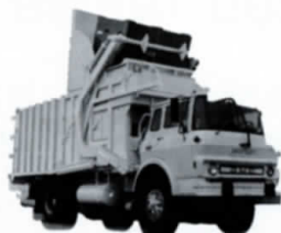
Container is lifted, rotated and refuse falls into body
