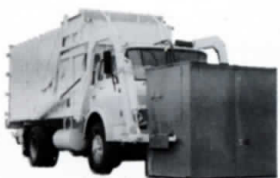
Lifting arms engage container
