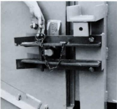
Container guides and locks on the PowerMite provide quick container hook-up.
