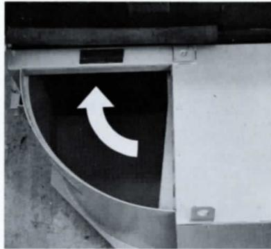
PowerMite's powerful packer head sweeps through the charging box, moving refuse into the container.
