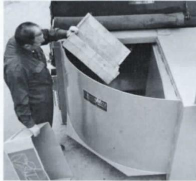
PowerMite's big charging box allows bulky boxes and large objects to be hand loaded from ground level.
