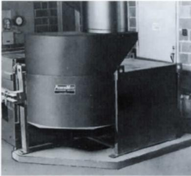
PowerMite may be chute fed or conveyor loaded. Optional hoppers are available to fit your needs.
