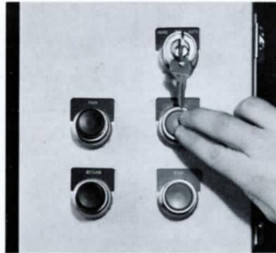
PowerMite is easy to operate. Push-button controls give manual or automatic continuous cycling.
