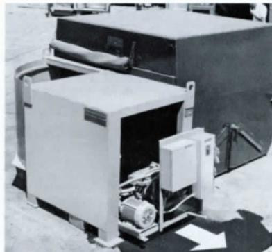
The self-contained power unit is skid-mounted for easy removal. It is mounted inside the packer for safe, tamper-proof operation.
