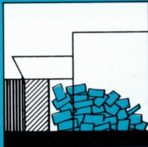
Packer plate sweeps material into attached container.
