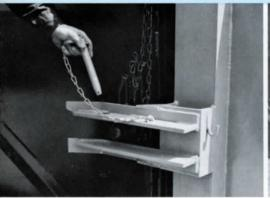
Combination container guides and locks on the sides of the PowerMite assure easy alignment with the Dumpster container. Container is securely locked to the packer by drop pins.
