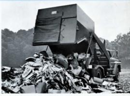
After PowerMite compacts the refuse, the Dempster-Dumpster picks up the container and hauls it away. Special baffling inside container releases the tightly compacted material for easy dumping.
