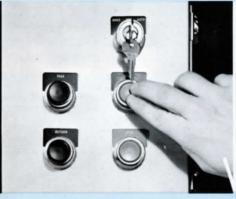
The control unit consists of a push-button panel with a three-position key-switch selector for manual or pre-programmed automatic cycling. Turn key to manual, for PowerMite's exclusive "Super Stroke" boost pressure.
