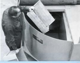
PowerMite can be loaded from the front or side from ground level. Low 52" charging box height makes loading easy.
