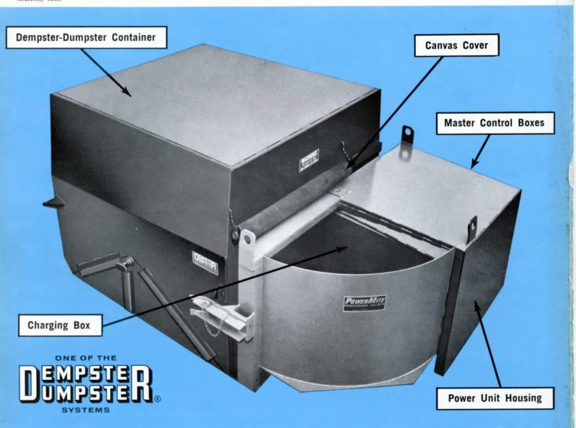
The PowerMite Stationary Packer is a small hydraulic packer which compacts refuse into a special Dumpster container or other types of large refuse containers. When container is full, a truck mounted Dempster-Dumpster picks up, hauls, empties and returns container to original packing position. Depending on the material, PowerMite can increase container payloads 4 times or more. PowerMite comes complete with a double-acting cylinder, power unit and container positioning guides and locks.
