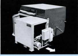
The self-contained power unit is skid mounted for easy removal or remote installation if desired. It's mounted inside the strong steel packer frame for safe, quiet, trouble-free operation.
