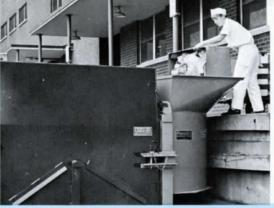
PowerMite can be placed flush against a loading dock. No special dockboard is needed. Optional hoppers are available to fit various applications.
