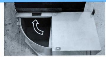
The sweep action of the packer head moves refuse from the charging box into the container. The double-acting hydraulic cylinder exerts over 42,000 lbs. of powerful thrust against the packer head, assuring tight, dense compaction.
