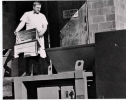
Optional hopper provides additional loading capacity and assures proper feed of refuse into packer.
