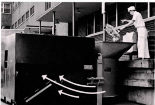
Baffling inside the container assures maximum compaction for large pay loads.
