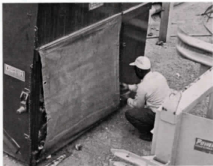
Tight fitting canvas cover is fastened in place to prevent spillage while container is enroute to the dumping site.
