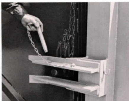
Container guides allow driver to position container next to the PowerMite without leaving the cab. Drop pins are secured for positive locking.
