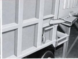
Automatic lock-hooks engage the trailer as it is backed into loading position. Hard rubber pads absorb shock of coupling operations.
