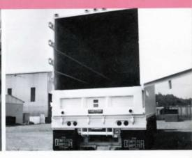
Doors of Refuse Transport Trailer are reinforced for maximum strength. Lower door prevents feed back and spillage of material . . . insures easy closure of top door.
