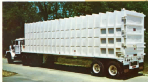
High tensil steel constructed Transport Trailer.
