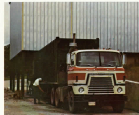
Refuse is chute fed into an economical SP78-90 Stationary Packer at a low volume Transfer Station.
