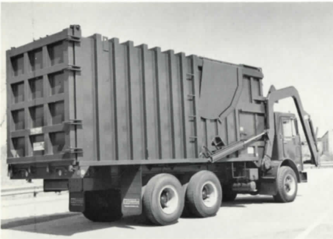
High Tensile Steel Body and tailgate is strong enough to withstand tremendous internal packing pressure. Rigid reinforcing on the side, top, and tailgate prevent distortion and bowing.
