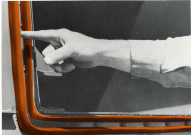
Heavy-Duty Rear Door Seal located around the inside perimeter of the tailgate, serves as an effective liquid seal. Improved gasket design with deep flanges assure more durability and longer life for retaining liquids inside the body.
