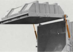
The top hinged Stor-Dor Tailgate is quickly opened by the action of two side-mounted, single-acting cylinders.
