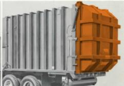
The Stor-Dor Tailgate is heavily reinforced with high tensile steel channels to withstand packing pressure. Neoprene gasket provides liquid tight seal.
