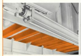
Rigid, closely spaced hat section reinforcing supports the floor for maximum strength, and eliminates "wash boarding".
