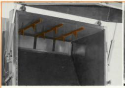
Three rows of material retainer teeth at the top of the body prevent fall-back of compacted material when the packer head is retracted.
