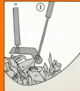
CRUSH: crushing material against hopper floor.
