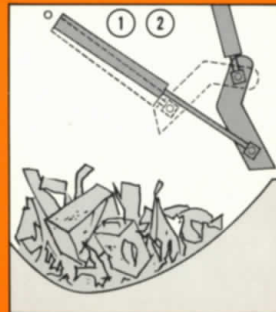
START: packing cycle begins as packer panel moves back.
