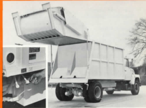
Ejector and Tailgate Lift Cylinder Controls Two hand control levers are located on the driver's side at the front of the body. One activates the two lift-cylinders which raise the tailgate. The other controls the ejector head. Manually actuated electric control maintains proper engine speed.
