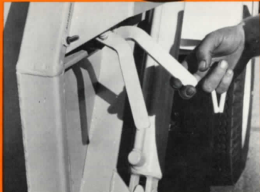
Split Cycle/Semi-Automatic Packing Controls Packing controls are on rear curb side of tailgate section. To start packing cycle, both packing levers are pushed downward. To complete cycle, controls are pulled upward. Manually actuated electric control maintains proper engine speed.
