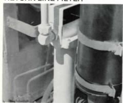
HYDRAULIC RETURN LINE FILTER keeps oil cleaner so it lasts longer. This efficient system extends the life of the hydraulics.
