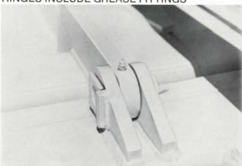
For extended life and reduced noise all hinges are equipped with grease fittings. The cylinder includes a knuckle for precise hopper cover adjustment.
