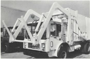
Dumpmaster's front loader arms have gross lifting capacities of 4,800 or 8,000 pounds. Heavy, self-packing containers can be handled with a minimum of strain and wear. The hydraulic loader assembly is activated inside the cab by easy-to-operate manual controls. Rugged box-type arm construction is designed for heavy lifting.
