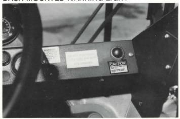
This warning light system meets or exceeds all ANSI requirements, by clearly indicating when the hopper cover is open, the tailgate is not fully closed or the arms are above the body.
