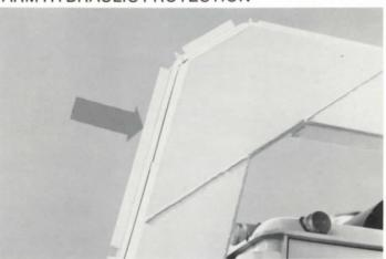
A steel bar running the length of both arms protects both feed and return hydraulic lines from low hanging limbs and other possible obstructions.
