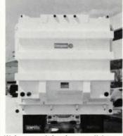
We've moved the clearance lights down so they're less vulnerable to tree limbs. Also, Dumpmaster's traffic signal lights have been moved up to prevent damage by refuse at the dump site.
