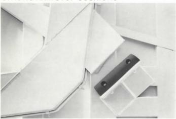
These heavy-duty rubber stops prevent arm over-travel and cushion the shock loads when heavy containers are dumped into the hopper.
