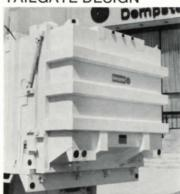
On 28, 34 and 41 cubic yard bodies. Reinforced with high-tensile steel channels to withstand high internal packing pressure, the Stor-Dor tailgate is top-hinged with manual rear-door latch. Two side-mounted single acting cylinders open quickly for material ejection.
