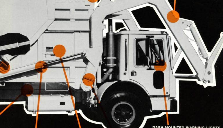
CHEVRON SHAFT PACKING FOR EASIER HYDRAULIC SERVICING CHROME PLATED HYDRAULIC CYLINDER SHAFTS DASH-MOUNTED WARNING LIGHTS MEET OR EXCEED ALL ANSI SAFETY REQUIREMENTS
