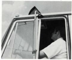
CAB-O-SCOPE mounted in cab ceiling allows operator to view containers during all stages of dumping process. Installs easily in the field or can be mounted at the factory.
