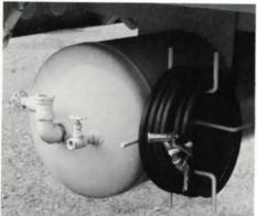
WASH-OUT TANK mounted under the rear of the body holds water or liquid deodorant compound. Connected to the truck chassis air supply system, the pressurized wash-out system permits quick and convenient cleaning of containers.
