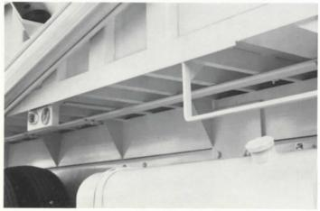
The 9" body longitudinals are mounted directly to the chassis frame eliminating the need for wood stringers. %-inch high-tensile steel floor with three-inch structural channel crossmembers provides extra strength and longer life.
