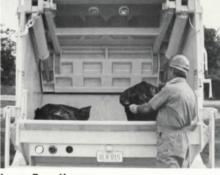
The low-profile, deep hopper holds 3 cubic yards by swept volume. The low loading height and deep well hopper reduce loader fatigue and the number of packing cycles required.
