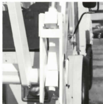
Fork assembly Fork shaft mounted in split bearings for ease of maintenance.
