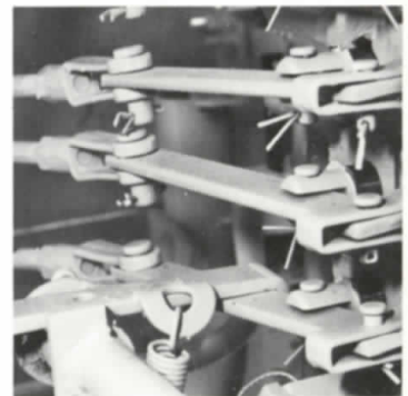
Dump arm limit device Mechanical device which makes it impossible to dump containers until packing blade is in the full forward position.
