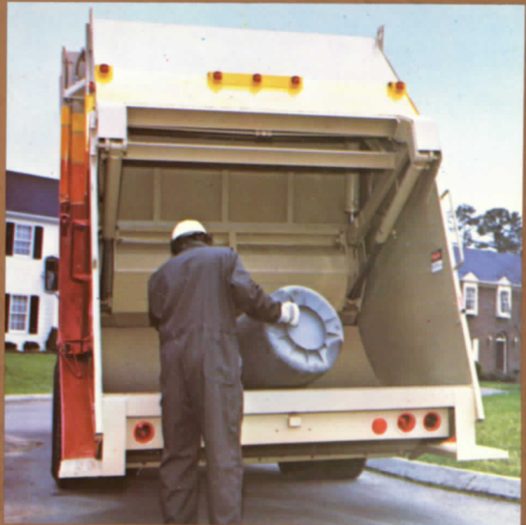
Large 3 cubic yard hopper increases loading efficiency. TBEA rated, largest on any mid-range. Full 80" wide, with low loading height.
