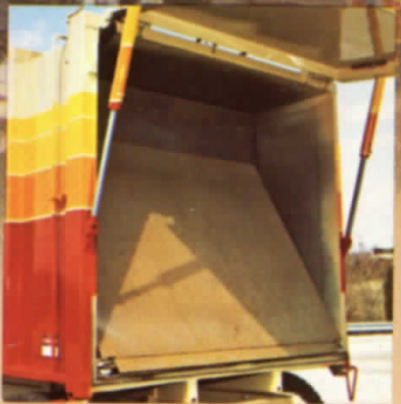
Face of ejector panel is completely smooth. There are no obstructions or "dog house", entire load falls free.
