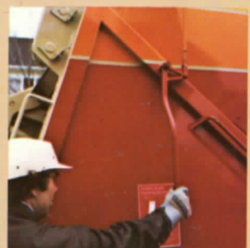
Large 3 cubic yard hopper increases loading efficiency. TBEA rated, largest on any mid-range. Full 80" wide, with low loading height.
